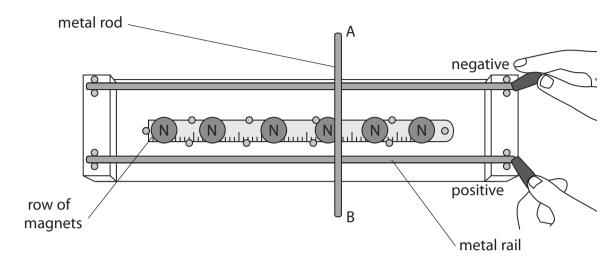
The student connects the two parallel horizontal metal rails to the positive and negative terminals of a power supply.
