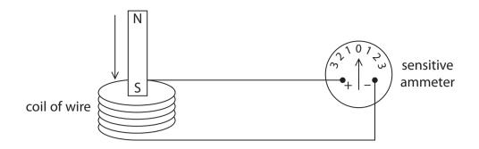
When the S pole of the magnet is moved into the coil, the pointer on the sensitive ammeter moves to the left.
