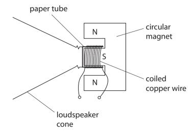
A coil of wire is wrapped around a paper tube attached to the loudspeaker cone.
